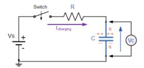
The charge Q on the capacitor is related to the current I by dQ/dt=I. Furthermore, by Kirchhoff's law, V-RI-Vc=0, and the charge Q on the capacitor is Q=CVc, where C is the capacitance. That can be combined to give the differential equation
