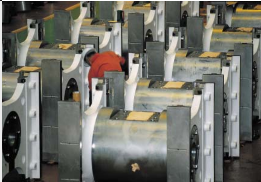
Crosshead pins with guide shoes for Sulzer RTA96C engines.
