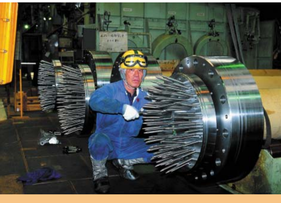
Cooling oil spray nozzles at top of piston rod
