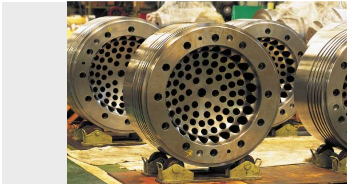
Bore-cooled pistons from the underside.
