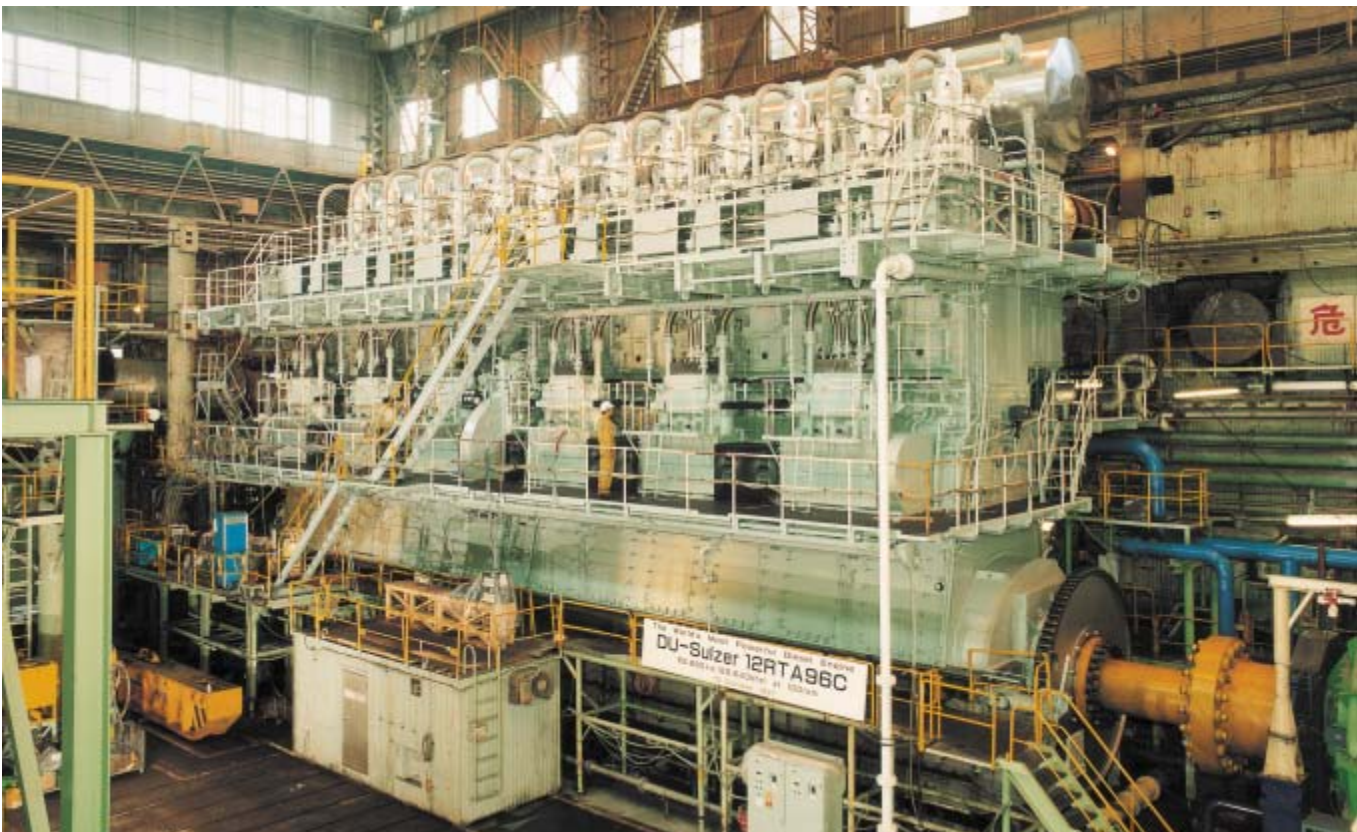
12-cylinder Sulzer RTA96C engine giving 68,640 kW (93,360 bhp)
