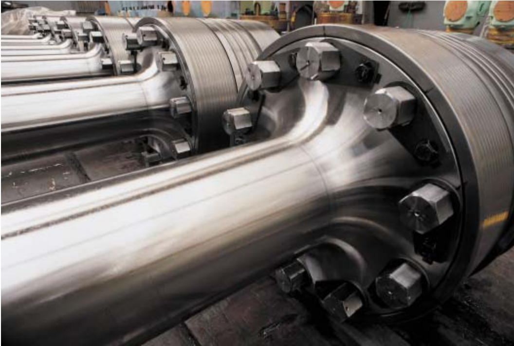
Pistons of Sulzer RTA96C engines
